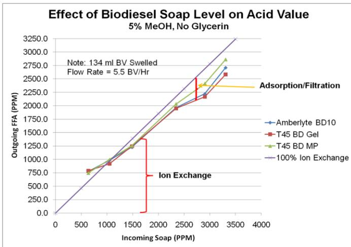
The straight line on the graph represents an ideal ion exchange curve, where all of the soap entering the column of beads is converted to free fatty acids. It is apparent that at soap levels above 1,000 ppm, the free fatty acids in the effluent biodiesel are lower than the predicted amount, even though the soap was removed from the biodiesel. Therefore, some other modes of cleaning must have been operating in addition to ion exchange.
