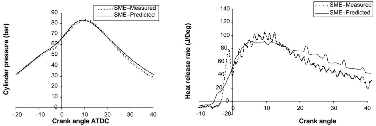
Figure 2. Measured and predicted cylinder pressures and heat release rate for SME.
