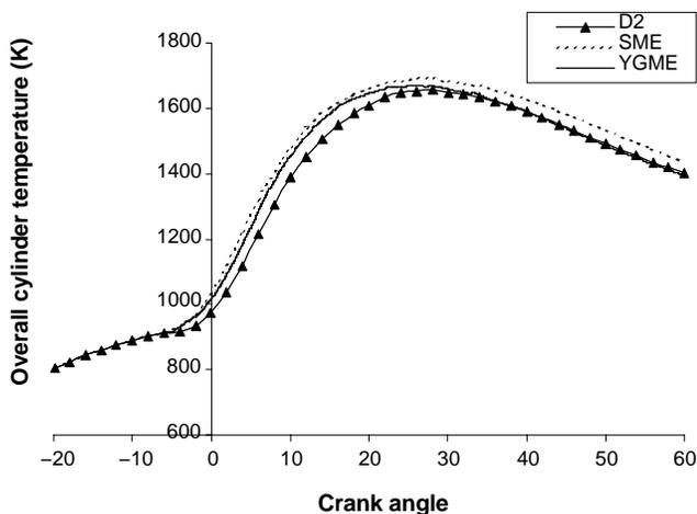
Figure 7. Overall cylinder temperatures of D2, SME, and YGME.
