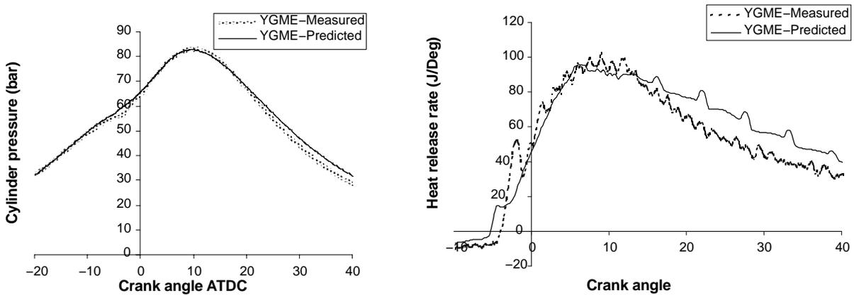
Figure 3. Measured and predicted cylinder pressures and heat release rate for YGME.
