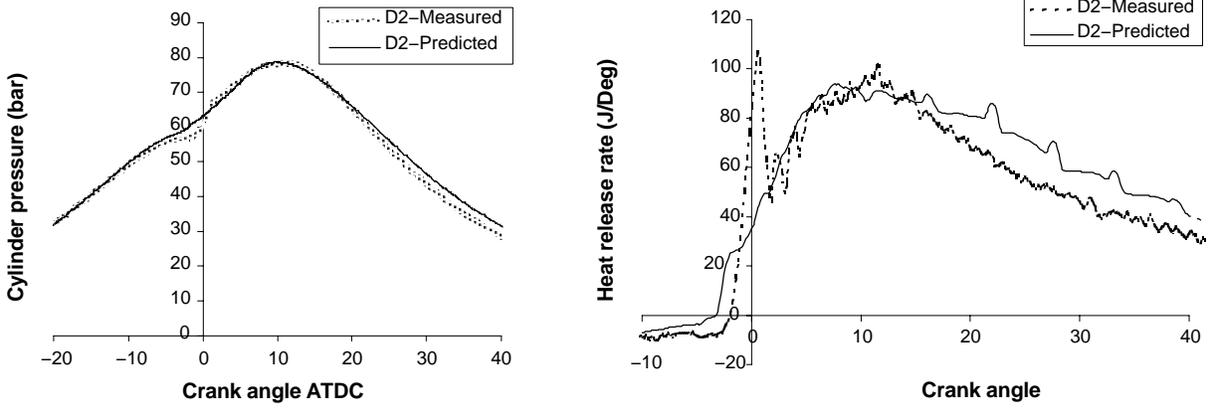
Figure 1. Measured and predicted cylinder pressures and heat release rate for D2.
