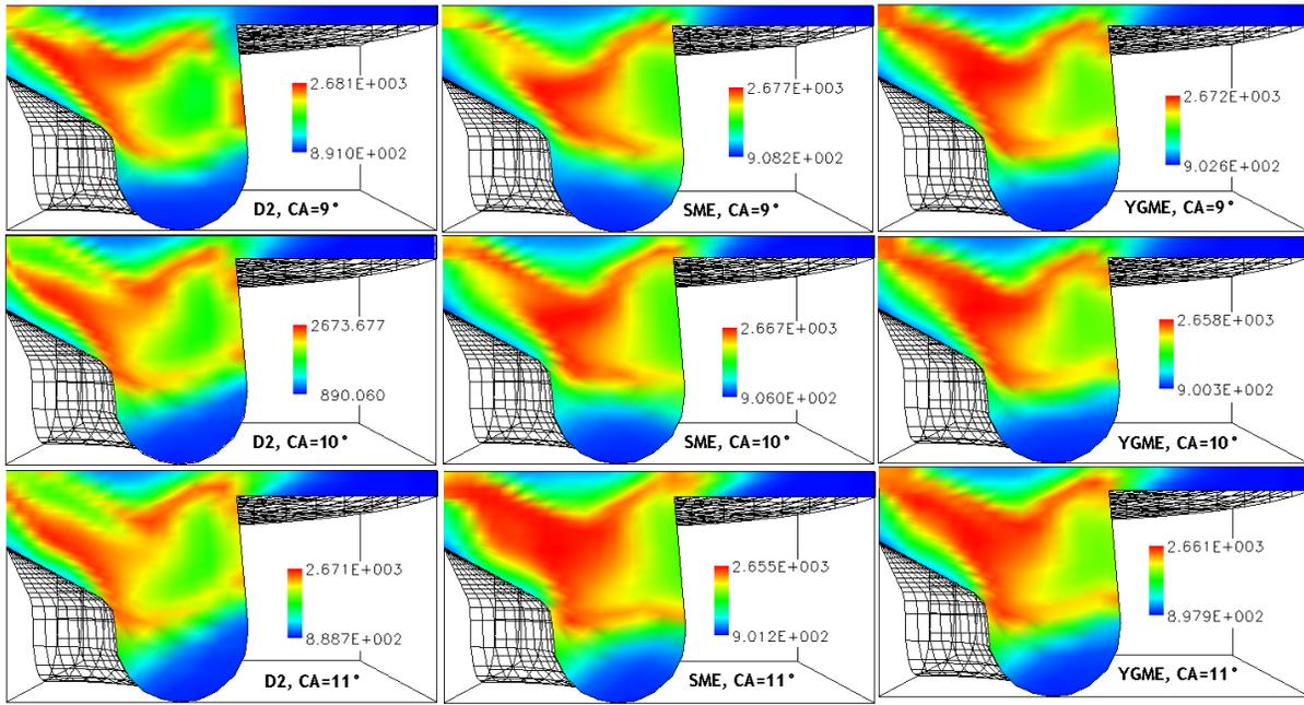
Figure 6. In-cylinder temperature distributions of D2, SME, and YGME (from left to right) at crank angles of 9°, 10°, and 11° (from top to bottom) at  $y = 0$  plane.
