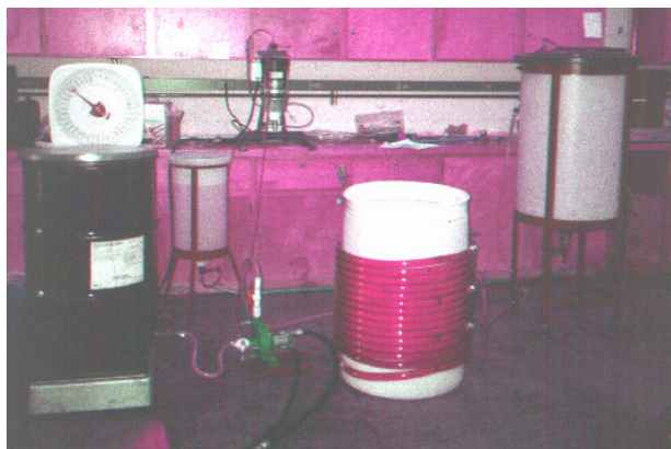
Figure 3. Continuous flow system (CF-1). The first attempt at a reactor for the continuous flow system. It consisted of about 30.5 m (100 ft) of 25.4-mm (1-in) clear polyvinyl chloride tubing in a helical pattern. Also shown in this picture are the centrifugal mixing pump to the left of the reactor and the FMI metering pump on the shelf to the left and rear of the reactor.
