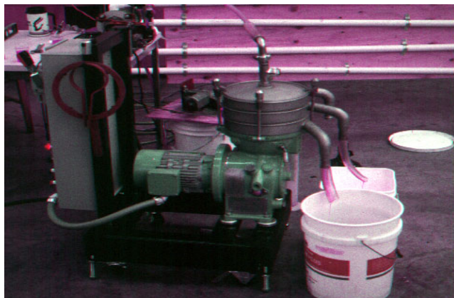
Figure 4. Alfa Laval model WSB 103B-74-60 continuous flow centrifuge used for ester and glycerol separation.
