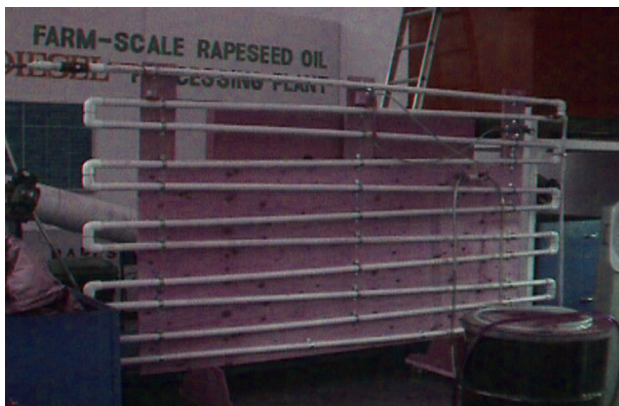
Figure 5. “Ladder type” retention reactor used in the final design for the continuous flow biodiesel production system. The reactor consists of 33.5 m (110 ft) of 31.8 mm (1 1/4-in) PVC arranged in 11 steps with 1.8 m (6-ft) of 22-mm (.5-in) PVC vertical exit section. Nine feet of clear PVC lines with static mixers used in the feed and exit lines are not visible.
