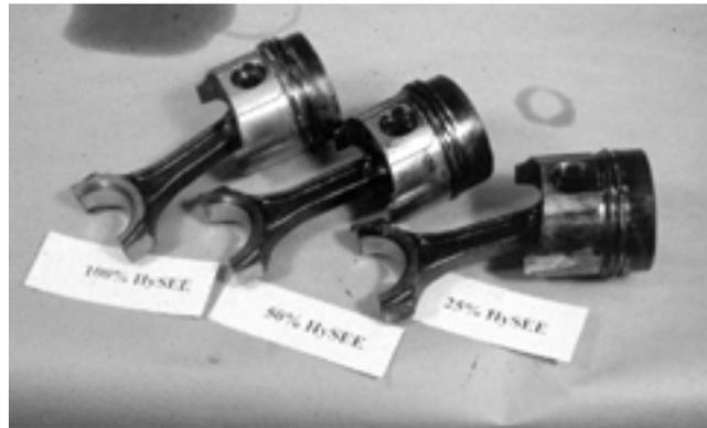
Figure 11—Pistons showing the relative amount of staining and deposits. From left to right are 100% HySEE, 50% HySEE, and 25% HySEE.
