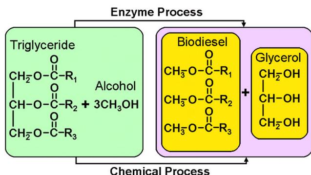
Figure 2. The transesterification reaction (Knothe et al. 2005). R<sub>1-3</sub> represents various fatty acid chains. The alcohol used for producing biodiesel is usually methanol.
