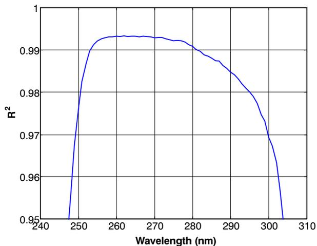
Figure 3.  $R^2$  of linear relation of biodiesel percentage and absorbance as a function of wavelength.
