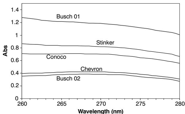
Figure 4. Absorbance of diesel diluted in *n*-heptane. Curves are marked with the name of the local gas stations where the samples were obtained. Busch01 and Busch02 were from the same station at different times of the year.
